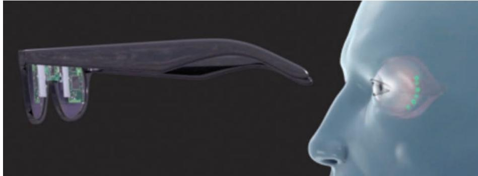
**A conceptual drawing of the Bionic Sight neuroprosthetic device that is built into a pair of glasses or goggles and relays signals to retinal ganglion cells injected with a transgene to restore vision in people with damaged photoreceptors.**
