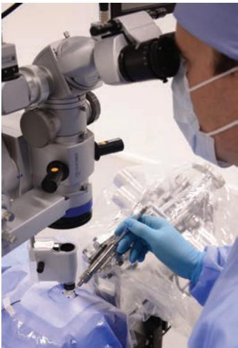
This surgical robot guided a 0.03-mm needle into the occluded retinal vein.
